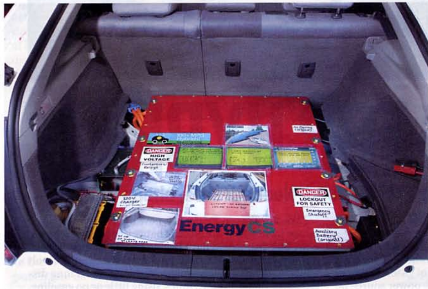
Kramer's converted hybrid uses lithium ion batteries with an additive to quell overheating.
