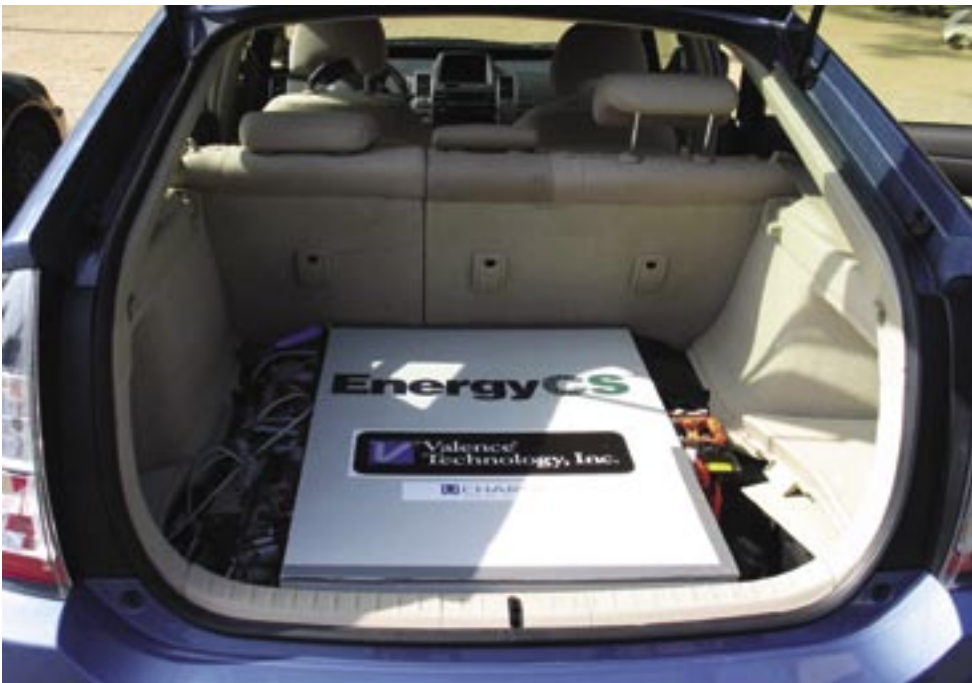
Saphion lithium-ion batteries used in this plug-in hybrid are positioned in the rear cargo area.
